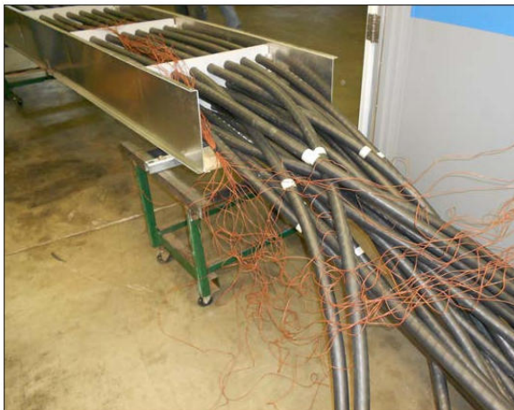
ABOVE—A temperature rise test being run on an Abcope Cable Bus system.
